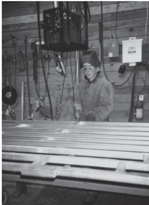
**Photos:** (1- welding without gloves or jacket, 2-getting ready to weld with all proper safety equipment)
